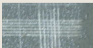
Ancamide 2652 12 weeks exposure Recoatibility = 10
