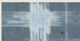
Standard Polyamide 12 weeks exposure Recoatibility = 1
