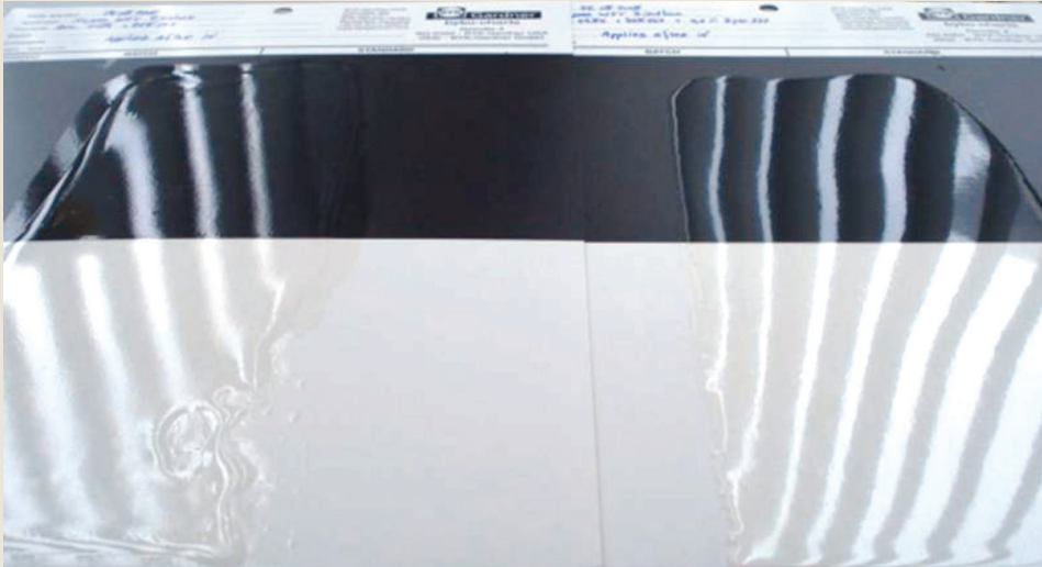
FIGURE 6: APPEARANCE OF 75 µ CLEAR COATS APPLIED WITHOUT ADDITIVES (LEFT) AND USING A LEVELING ADDITIVE (RIGHT), FOLLOWING A 10 MINUTES INDUCTION TIME. ANCAMINE 2685 CURING AGENT WAS MIXED AT 48 PHR WITH A BIS-A/F EPOXY RESIN DILUTED WITH EPODIL® 748, EEW195, µ 900 MPA.S
