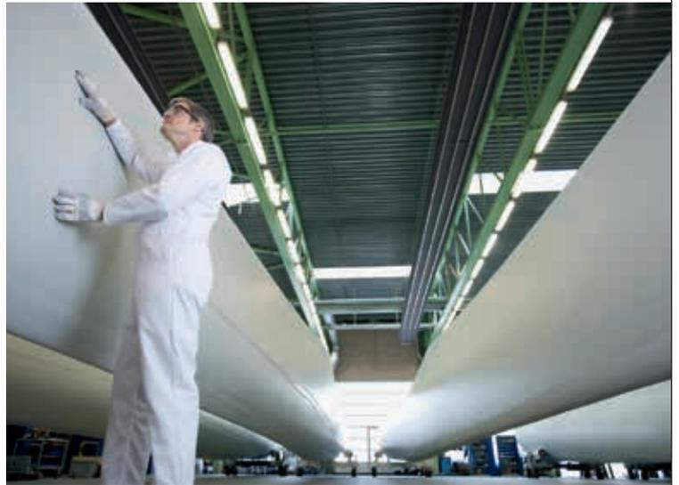
**PRECISION WORK ON A GRAND SCALE:** Before a rotor blade leaves a manufacturing facility, it is examined closely for defects and cracks. Even minor material weaknesses can lead to costly breakdowns during peak-load operations
