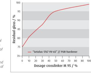
Figure 4: Residual gloss after modified scratch test of a 2K PUR system formulated with PUR-hardener and additional levels of crosslinker M 95
