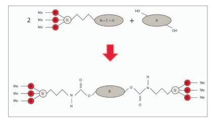
*Figure 1: IPMS-based silane-urethane hybrid crosslinker containing urethane groups, terminated by tri-functional alkoxy-silane structures*
