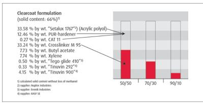
*Figure 3: Example of a clearcoat formulation with 50:50 pbw (on solids) of resin/ PUR-hardener and crosslinker M 95*
