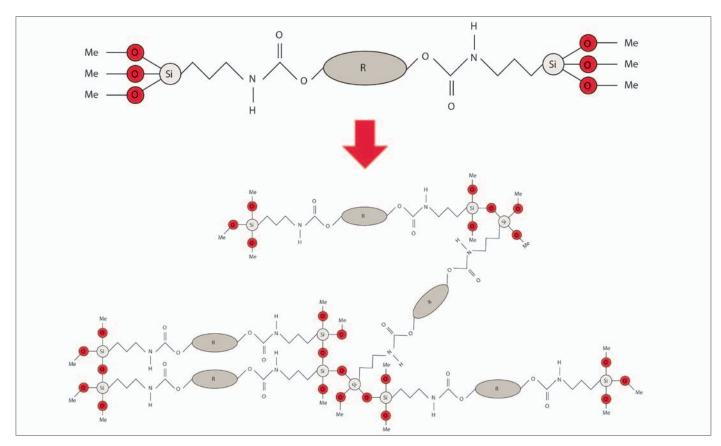
Figure 2: Hydrolysis-condensation reaction forming siloxane networks
