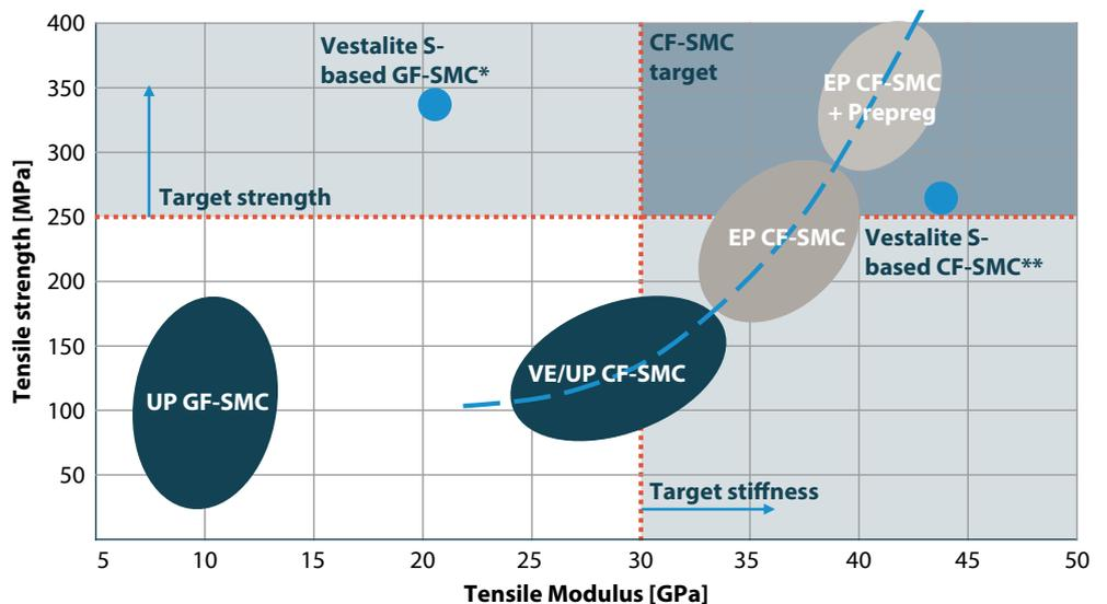
FIGURE 3 Comparison of mechanical properties of different SMC systems with the Vestalite S coefficients, based on the material characterization at the Fraunhofer ICT (© Vestaro)
