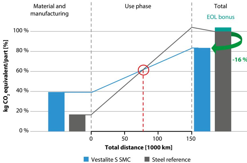
FIGURE 5 Results of the life cycle assessment for the steel-based and Vestalite S-based SMC tailgate as part of the project (© Vestaro)
