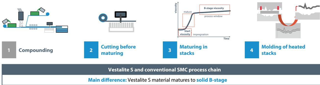
FIGURE 2 Sample Vestalite S process chain (differences from conventional SMC processes shown in blue) (© Vestaro)
