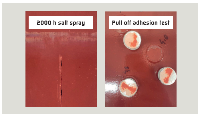
Figure 4: Anti-corrosive primer system based on “Ancamine 2739” after accelerated weathering and pull-off adhesion test.
