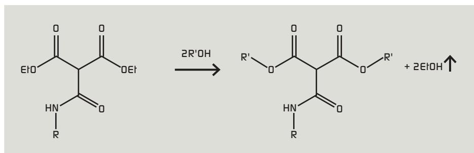
Figure 4: Functionality of blocked PUR crosslinkers for powder coatings.
